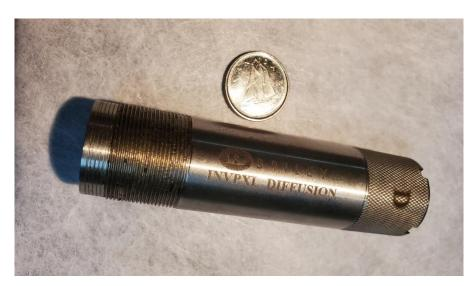
Often called a "Spreader" choke (S), sometimes referred to as a "Diffuser" choke (D) this is a choice for skeet's low targets that are coming towards you, sporting clays' rabbit and some springing teal targets. A negative choke has an inside diameter greater than the barrel's bore. To help achieve this greater diameter, negative chokes often extend beyond the muzzle. Patterns open fast and wide, making it easier to connect on "up close and personal" targets.
