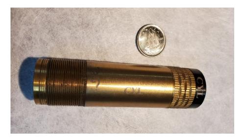
A Cylinder choke (C) has no constriction, the inside diameter is the same as the shotgun's bore. The absence of constriction means patterns open up very quickly. Cylinder works well on close skeet targets like at Station Eight or low–house birds at Stations One and Two. This choke allows for a rapidly expanding pattern and will help you to hit targets described above or even the pesky bouncing rabbit target in sporting clays.
