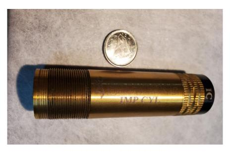
This is one of the more common choke constrictions, Improved Cylinder (IC) is a choke often carried by shooters and used by many. This choke is used for everything from 16—yard trap to the second shot on skeet pairs. It also works well on many of the clay target presentations thrown on the sporting clays course.
